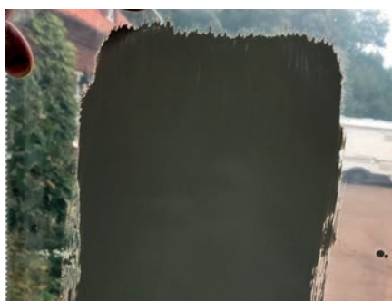
One coat should cover fully when viewed against the light. Approx. 100 microns.
