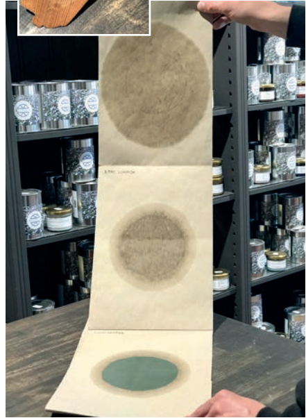
Painting on absorbent surfaces. There is a simple test to check the penetration of the paint/oil and the level of protection.
